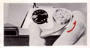
Advance the film with the advance lever and press the shutter release button. Do this twice. To be sure that the film is advanced by the film advance lever, seeing to it that the film rewind knob is also turning counter-clockwise.
