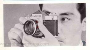
While looking through the viewfinder, turn the Focusing Ring either clockwise or counter-clockwise until a clear, distinct image is seen in the center microscreen spot.
