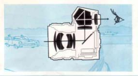
Viewing and focusing are both done through a single window.
