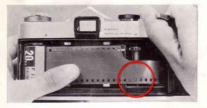
Position the film perforations over the teeth of the Take-up Spool Sprocket and pull the film taut by slowly moving the Film Advance Lever.
