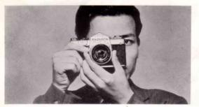
It is very important to hold your camera correctly and steadily when taking pictures in order to obtain good results. Hold it closely to your face with your elbows held close to your waist, so that blurring will not occur. The left shows how to hold your camera at a horizontal position.
