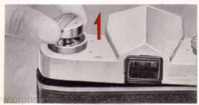
The Film Rewind Knob can now be pulled out to open the back of the camera.
