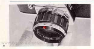
Turn the inner ring of the lens barrel, Aperture Control Ring, to the desired stop.
