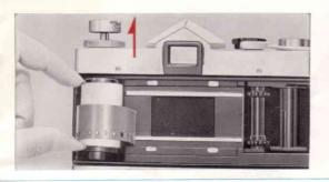
Pull out the Film Rewind Knob further and insert a roll of 35mm film in the film chamber. Then push the Film Rewind Knob back to position.
