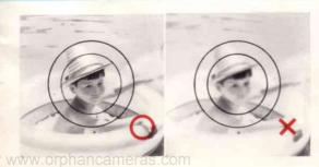
Viewing, focusing and picture taking are all done through a single window. You have only to bring the subject into clear focus by rotating the focusing ring and snap the picture.
