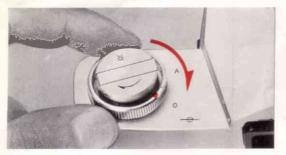
To unlock the back cover, turn the Release Dial to the direction of 'O' position.
