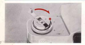
Close the Back Cover by pressing it with your fingers until it locks into position. And slide the Back Cover Release Dial to the direction of 'A' position.
