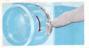
If you push down Aperture Opening Lever, the aperture is fully open and subject is clearly visible through the pentaprism viewer.
